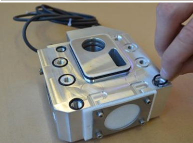
Fig. 3.6.10 Remove back plate O-rings [1211E], [1212E], [1213E].
