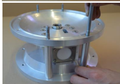
Fig. 3.6.2 Take out pin screws [14] and take care of the bushings [1204E]
