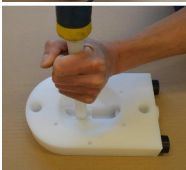
Fig. 3.4.4 To remove the spacer sleeve [19], use a plastic rod and a hammer to knock it out. NOTE! Be careful not to deform the spacer sleeve.
