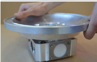
Fig. 3.6.9 Lift the diaphragms back plate [1201E].
