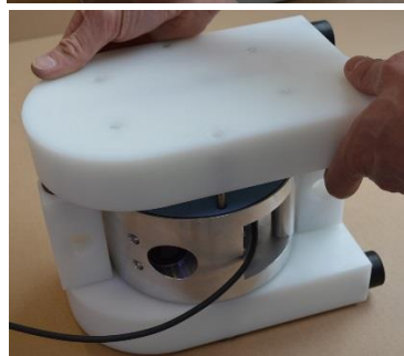
Fig. 3.4.2 Lay down the pump on one side and lift one of the housings [11].
