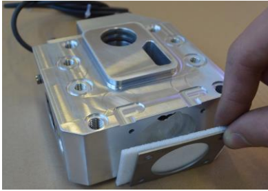
Fig. 3.6.13 Take out the muffler [25E] together with retaining plate [251E].
